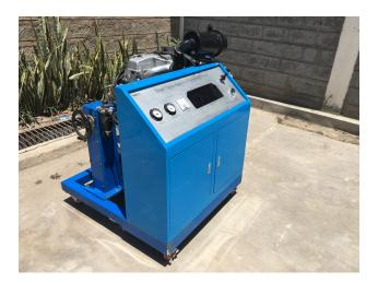
Figure A2: Noise Generating Engine
